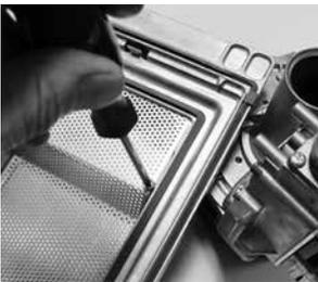
Removing gas air dividing plate
